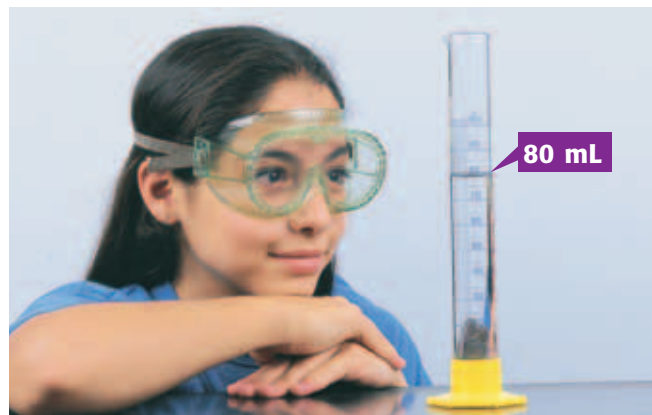
Figure 3 Adding a rock to a graduated cylinder raised the level of water from the 70 mL mark to the 80 mL mark. Because the rock displaced 10 mL of water and 1 \text{ mL} = 1 \text{ cm}^3 , the volume of the rock is 10 \text{ cm}^3 .
